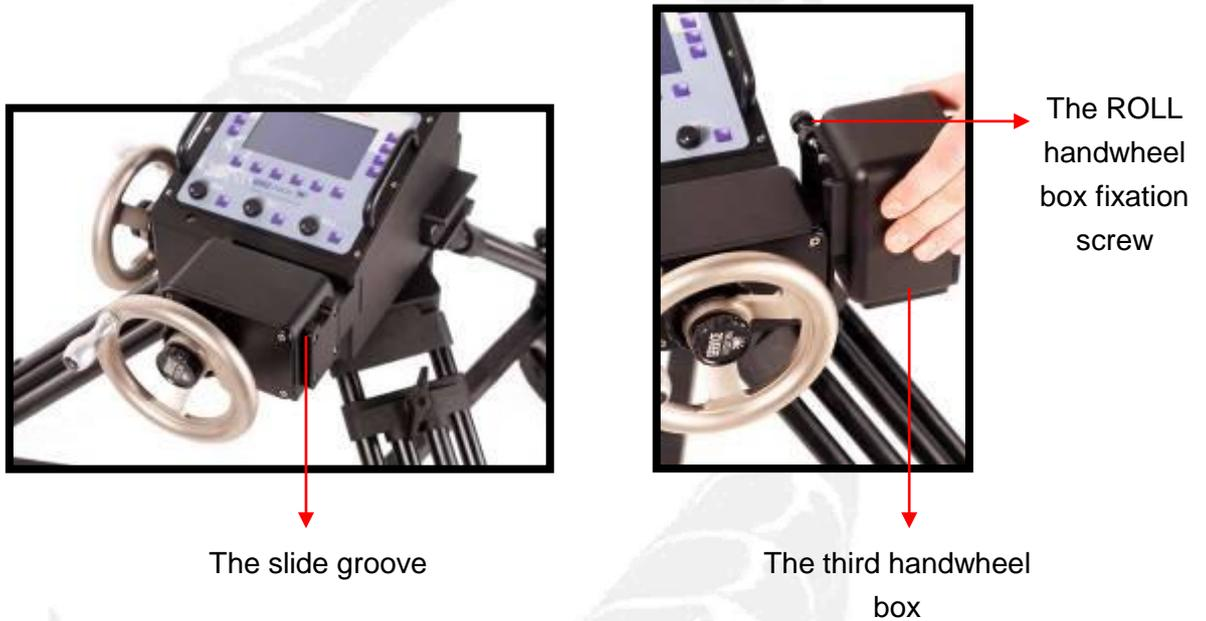
Lastly, the third axis box is connected to the ROLL HANDWHEEL connector.
